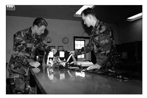
At left, A1C Scott A. Wold and SSgt. Dale E. Ludwig inspect an ejection seat's parachute and harness system. Regular and detailed inspection is important to make certain this equipment works as expected. The specialists in the survival equipment shop perform detail work that may go unnoticed—until an aircrew finds itself in an emergency.
