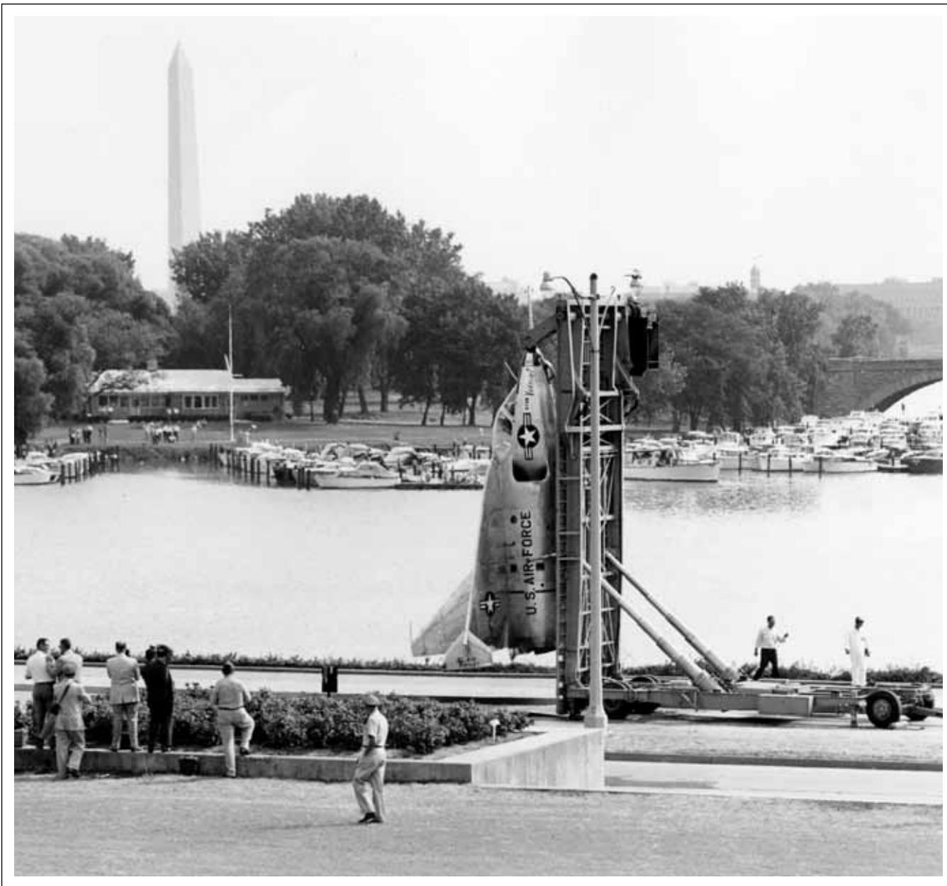
Two Ryan X-13 Vertijet research aircraft were built for the Air Force in the mid-1950s, expanding upon a 1947 Navy request to study a vertical takeoff and landing fighter that could operate from small ships. By the time Ryan test pilot Pete Girard demonstrated this pioneer VTOL aircraft (shown here) near the Pentagon in 1957, the small jet had made several successful flight tests. The X-13 had two small
