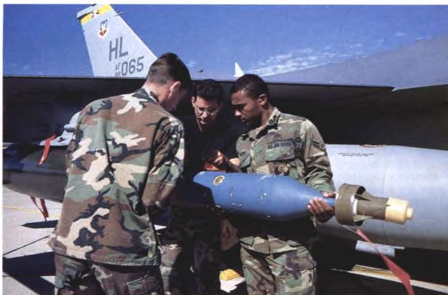
On the flight line, the weapons load crew works with the flight-line crew to load the weapon. Above, A1C Jamaal Brown drives the "jammer" as weapons load crew chief SSgt. John Barriball checks the 2,000-pound bomb. At right, once it's moved into position on the aircraft, load crew members (left to right) A1C Timothy Smith, Barriball, and Brown attach the guidance package that will turn the "iron bomb" into a GBU-24 precision guided weapon.
