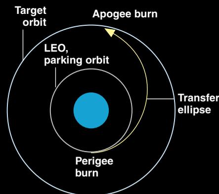
It is common procedure to pick an initial "parking" orbit, usually at LEO, then boost payloads to higher altitude. Engines are fired first (at perigee) to reach the apogee of an elliptical transfer orbit and then are fired again to put the spacecraft into a circular orbit at that higher altitude.
