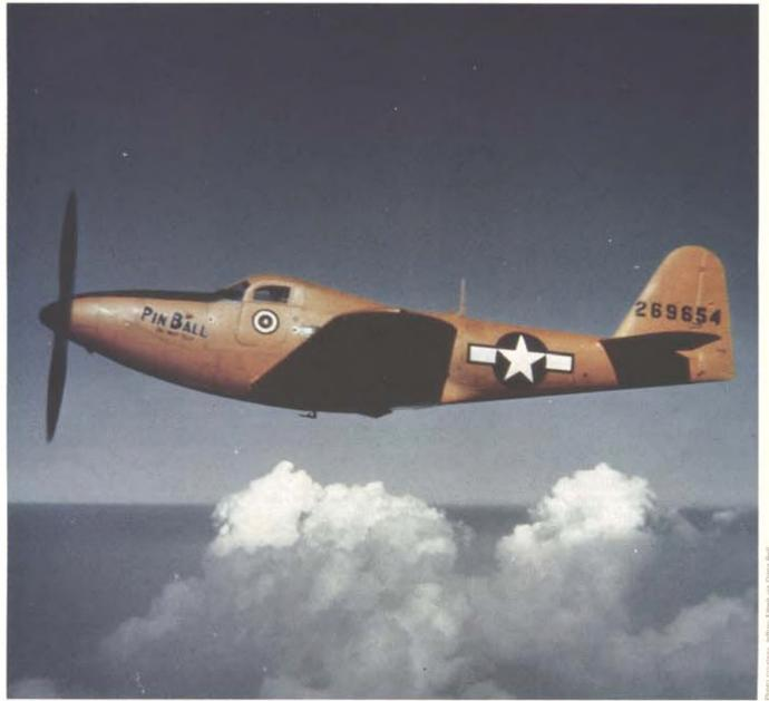
In 1943, Bell extensively modified a P-63 Kingcobra to serve as a target for bomber gunner training. All weapons and interior armor were removed, thicker metal sheet replaced the skin, the canopy was armored to protect the pilot, and more than 100 microphones were buried in the skin. A light in the propeller hub—and, later, additional
