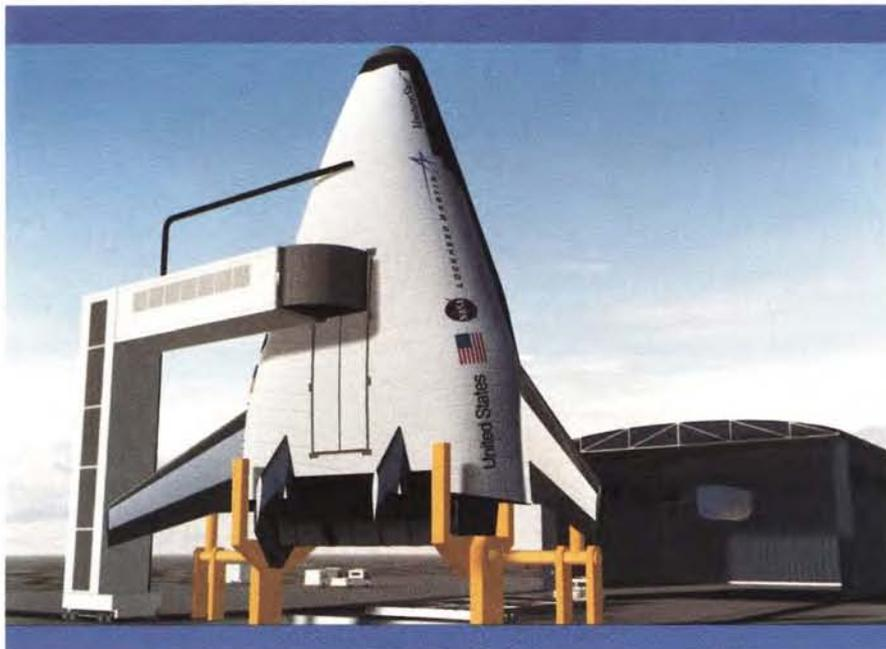
*In July, NASA selected Lockheed Martin to build the reusable launch vehicle X-33. The company's winning design, Venture Star (shown in this computerized visual), is expected to have a four- to seven-day turnaround time, with payloads of up to 40,000 pounds, and an on-time reliability rate of more than ninety percent.*
