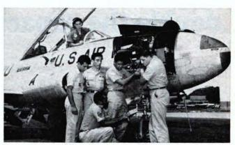
Uruguayan Air Force personnel at USAF School for Latin America train as flight-line radio repairmen on both pistonengine and jet-aircraft radio systems. Here bilingual in-structor demonstrates use of multimeter to check out T-33 communication system. After graduation, Uruguayans will become electronic specialists for units back home.
