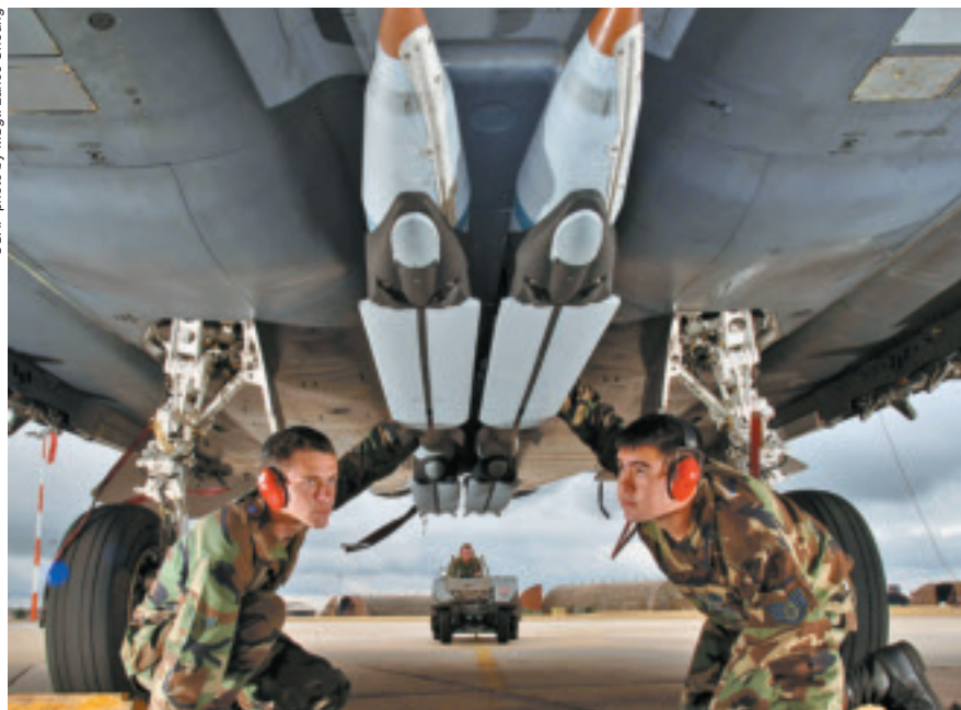
A1C Matt Aggers (l) and SSgt. Randy Broome check the stowed wings on ground-training Small Diameter Bombs loaded on an F-15E. The Air Force Operational Test and Evaluation Center was at the time evaluating the SDB weapon system.
