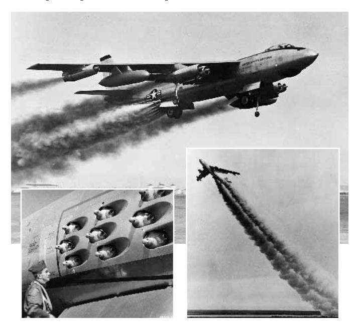
Boeing's swept-wing B-47 Stratojet of the late 1940s and 1950s could be a sight to behold. Clockwise from top: a late model B-47 on a JATO—Jet-Assisted Takeoff—flight; an XB-47 on one of the first JATO tests; and Maj. James Gallagher, a SAC pilot, inspecting installation of JATO bottles. Early jet engines lacked adequate thrust at low speeds, so B-47s were augmented with the JATO system, which added thrust
