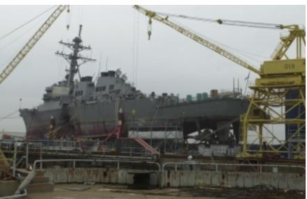
USS Cole during repairs aboard a Norwegian drydock vessel at a shipyard in Pascagoula, Miss.
