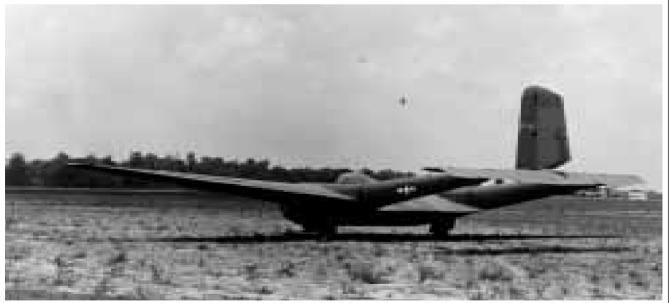
Sailplane and glider manufacturer William Hawley Bowlus began designing this flying wing glider, the XCG-16, in February 1942. It was a departure from the usual single-fuselage design of American gliders and introduced a twin boom. An early test flight of a full-scale model proved disastrous when it became unbalanced from weighted bags that were not tied down—the pilot and several passengers were killed.
