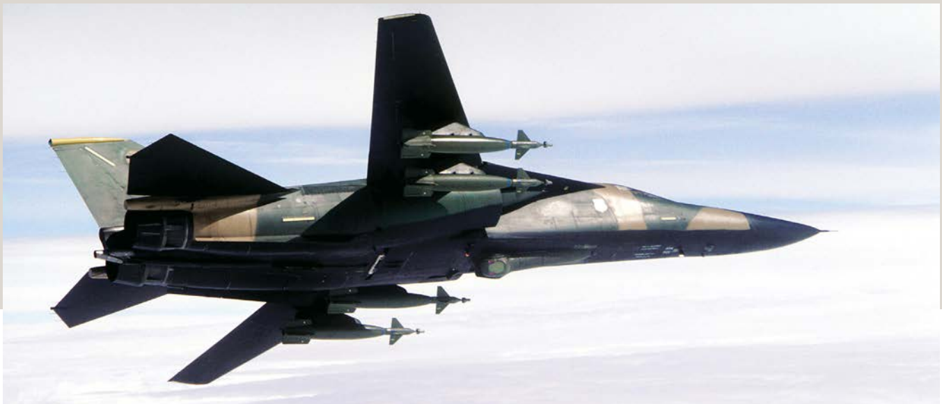
An F-111 carrying four GBU-10 Paveway II bombs and a Pave Tack laser target designator banks over Loch Ness, UK.
