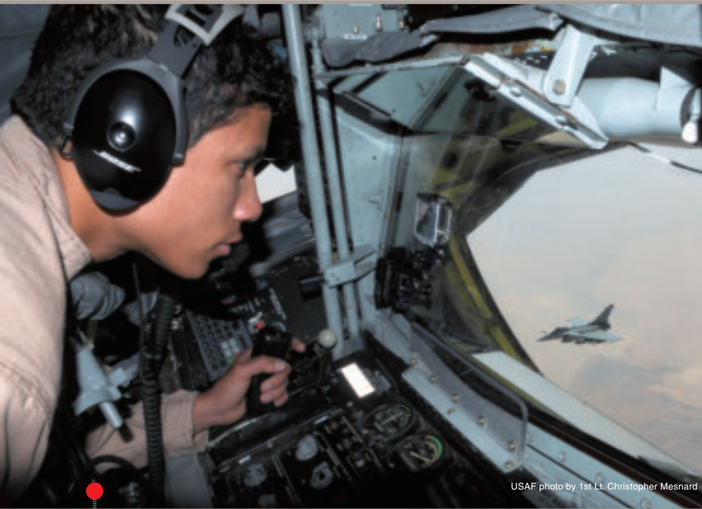
A1C Anthony Ellsworth extends the boom and drogue on a KC-135 as French fighters position for a refill.
