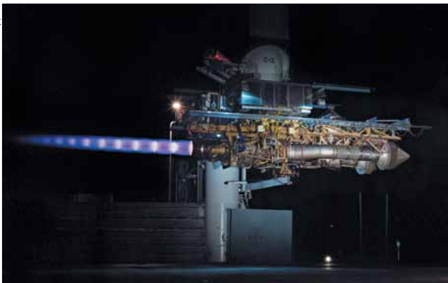
The F135 engine—shown here in a test—powers the F-35. It is a derivative of the F119 that powers the F-22, so it, too, has its origins in the 1990s.
