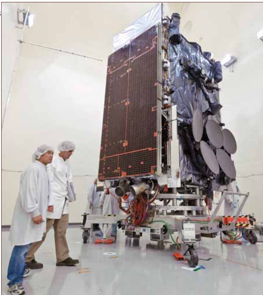
Technicians surround a Wideband Global SATCOM in the acoustic chamber at the Boeing satellite manufacturing facility in El Segundo, Calif. WGS satellites will serve as USAF's communications workhorses for some time forward.
