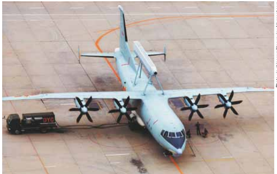
China's Y-8W/KJ-200 Balance Beam airborne early warning and control aircraft has a dual-sided active electronically scanned array radar mounted on top of a Y-8F-600 transport aircraft.
