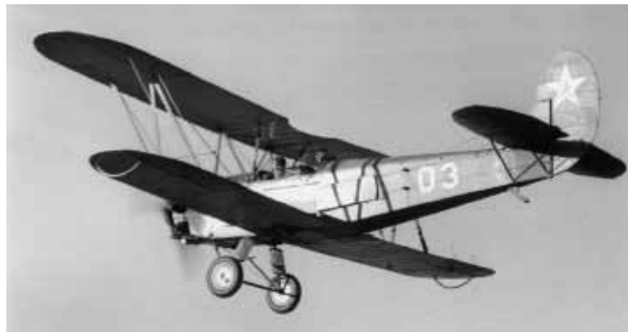
North Korean “Bed Check Charlie” attackers often flew the Polikarpov Po-2, such as this one in Russian military markings. The light biplane could fly low enough to hide among the ground clutter.
