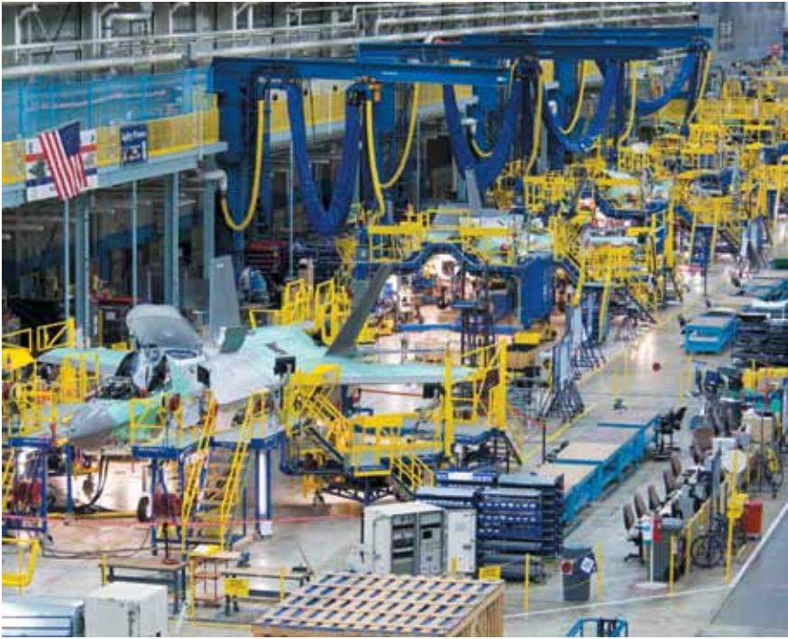
F-35s under assembly at Lockheed Martin's Fort Worth, Tex., plant. At planned peak, production will surpass 200 a year for US and allied air arms.
