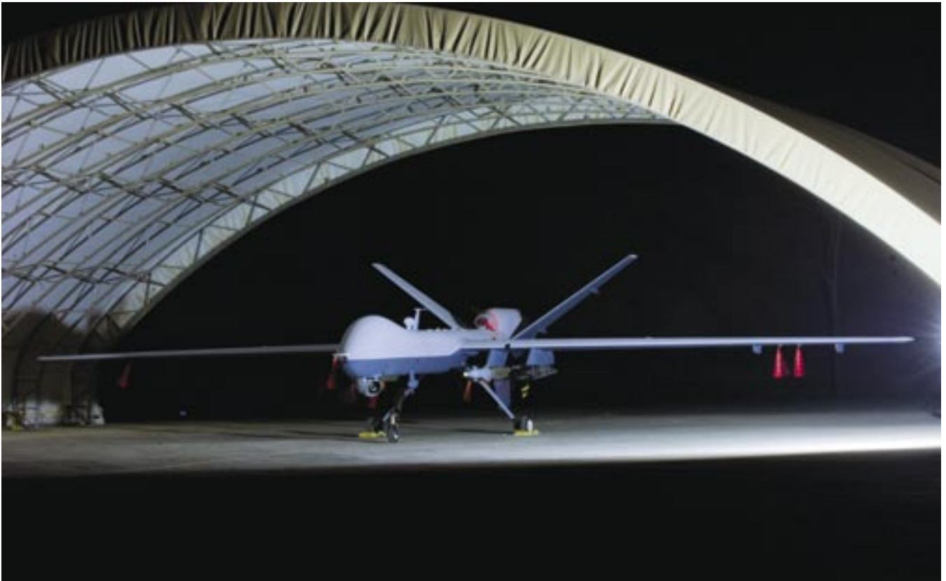
Heavy Duty: An MQ-9 Reaper is armed and ready for a mission at Joint Base Balad, Iraq. Larger and more powerful than its forerunner, the MQ-1 Predator, the Reaper can carry up to 3,750 pounds of laser guided bombs and Hellfire missiles. August marked the first weapons engagement in Iraq since it began flying combat sorties there in July.
