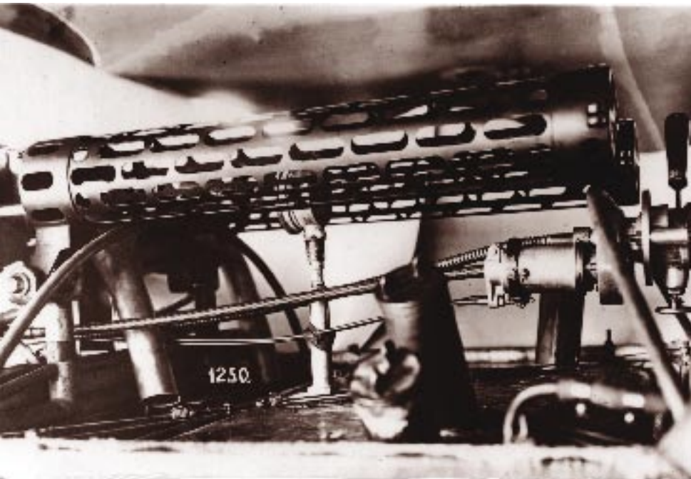
The synchronizer from a Fokker D-VII. German designer Anthony Fokker perfected the synchronizing system that Roland Garros had begun.
