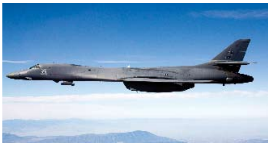
Targeting pods not only add high precision to legacy aircraft, they can turn them into prodigies of reconnaissance as well. Here, a B-1B sports a Sniper pod.
