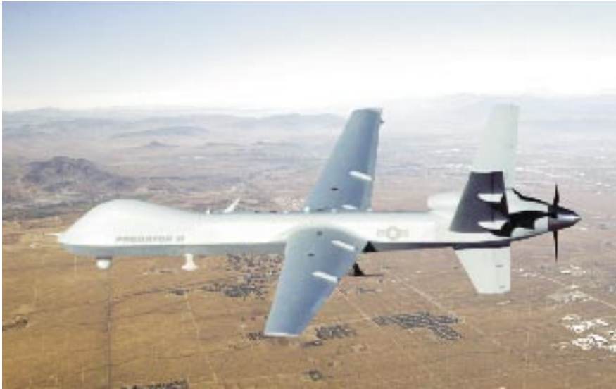
The MQ-9 Reaper can carry a battle load similar to that of the F-16 but stay in the target area upwards of 18 hours. The Air Force plans to buy up to 70 “hunter-killers.”
