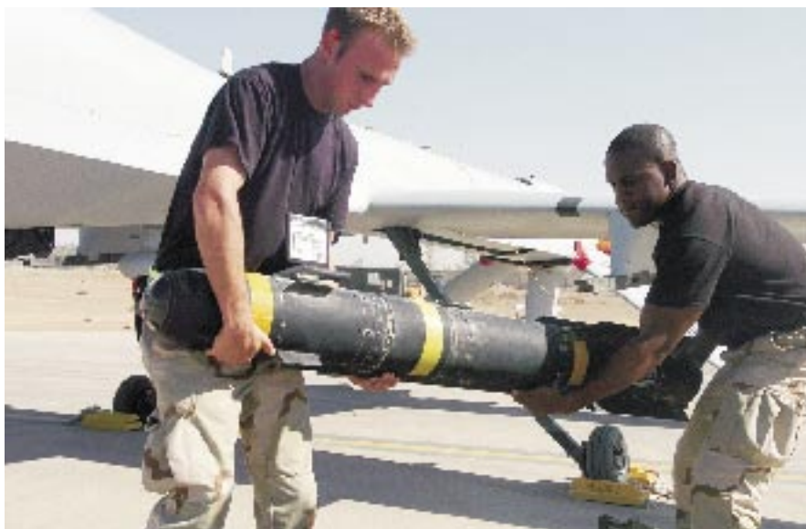
SSgt. Sean Pietre (l) and SrA. Rothschild Pierre-Louis III unload a Hellfire from an MQ-1 in Iraq.
