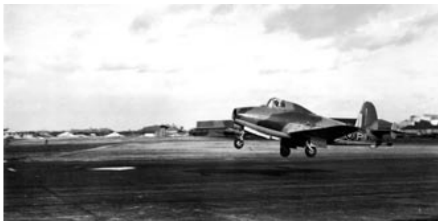
Whittle's Gloster E.28/39 was configured much like the He-178. The Gloster shown here on takeoff from Britain's Farnborough Testing and Evaluation Center is model # W4041/G. The G indicated that the aircraft was to be kept under armed guard at all times.
