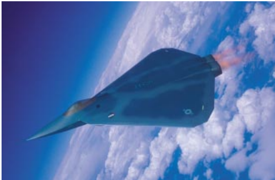
Lockheed Martin has done preliminary work on a tailless version of the F/A-22. Although this X-44 concept has not flown, USAF will consider such a configuration for the FB-22, if costs stay within bounds.
