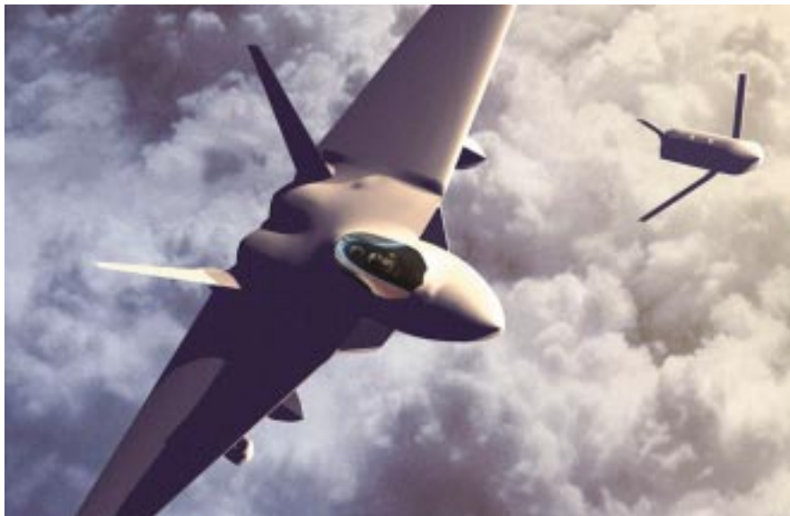
With missions of more than 15 hours, the FB-22 likely would have a two-pilot cockpit. The second pilot could spell the front seater and handle weapons management, as well as other missions.
