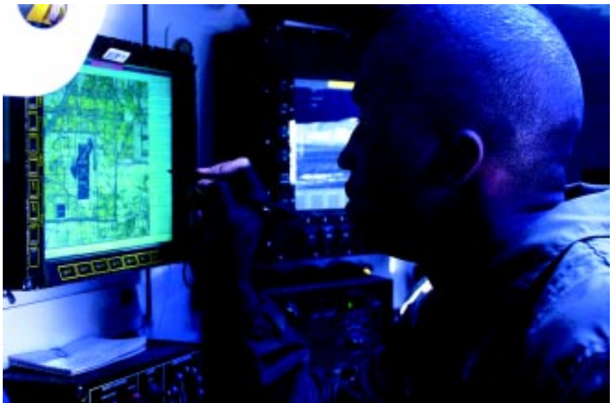
Tracking. Sgt. 1st Class Kenneth Dawson of Ft. Lewis, Wash., checks the map of his Force XXI Battle Command Brigade and Below (FBCB2) system, a widely used but limited blue force tracking system that is being improved.
