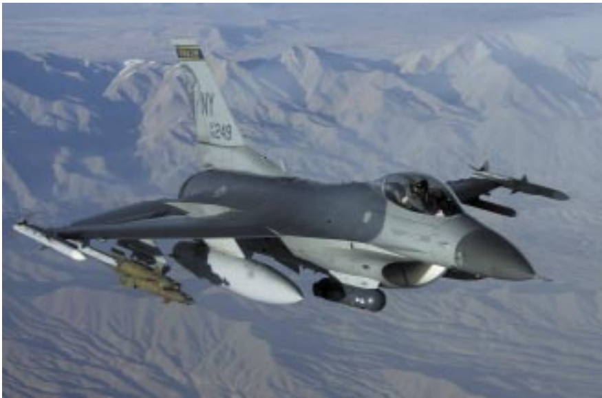
Over the years, F-16 equipment and armament have changed to keep pace with the threat. This New York Air National Guard F-16 flying over Afghanistan has a targeting pod and 500-pound laser guided bombs.
