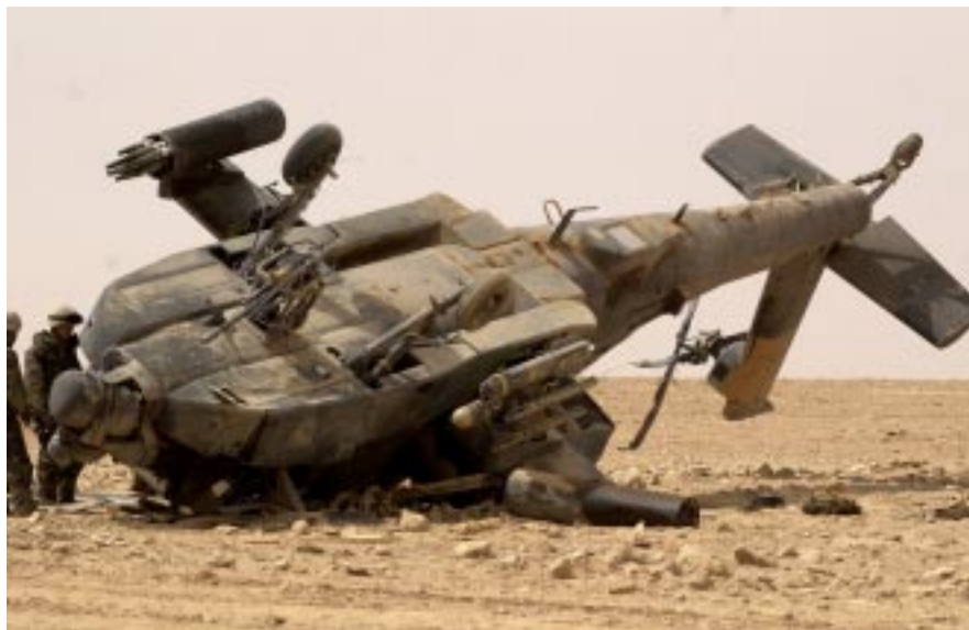
This AH-64 crashed during landing in Iraq on March 30. The Apaches suffered from mechanical problems and poor visibility caused by the fine dust of the Iraqi desert.
