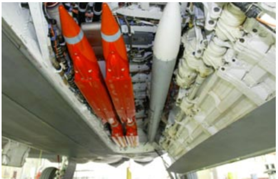
Small Diameter Bombs (red) likely will become the most ubiquitous ground attack weapons in the arsenal. Shown here in an F/A-22, the SDB will quadruple the number of targets each aircraft can hit on a single sortie.
