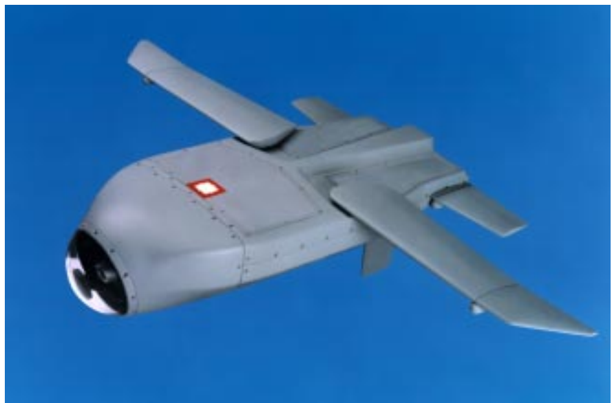
Smaller, smarter, and able to loiter—that’s the future of PGMs. Lockheed Martin’s tiny LOCAAS attacks in swarms and ignores targets other than its own. If it can’t strike its designated target, it destroys itself in air, avoiding collateral damage.
