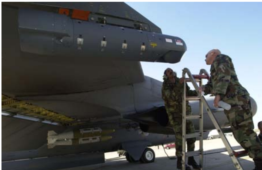
Old Horse, High Tech. A B-52 with a Litening II targeting pod put laser guided bombs on target close to friendly ground troops. Here, TSgt. Ken Williams, Barksdale AFB, La., and TSgt. Noel Peters, Luke AFB, Ariz., clean a pod's lenses.
