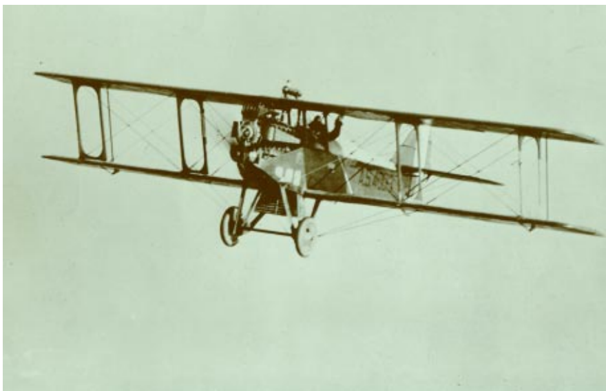
On Sept. 28, 1921, 1st Lt. John Macready set a world altitude record of 36,750 feet in this supercharged LePere aircraft, with a propeller designed for both “thick” and “thin” air.
