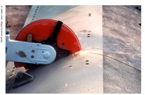
The INF treaty called for destruction of all but eight display articles. Here, at Davis-Monthan AFB, Ariz., a circular saw cuts through the door of a GLCM transport-launch vehicle.
