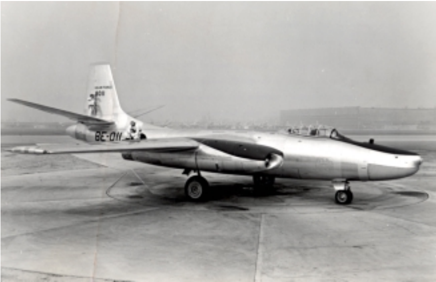
This RB-45C, a special version of the B-45 Tornado bomber, had five camera stations for its charting, mapping, and photoreconnaissance missions, which were carried out at high and low altitudes, day and night.
