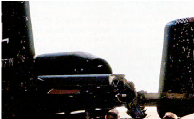
This close-up view of the tail section of a 23rd TFW A-10A aircraft from England AFB, La., shows the damage it sustained when an SA-16 missile exploded near it during Desert Storm.
