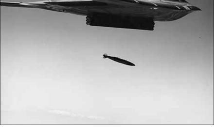
At top, a B-2 takes on fuel from a KC-135 during an Operation Allied Force mission. Above, a Block 20 B-2 uses the GPS–Aided Targeting System to guide a munition during testing. In Allied Force, the combination of the Block 30 B-2's GATS with the JDAM produced outstanding accuracy.
