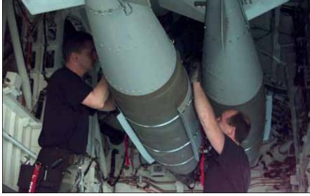
The other part of the B-2 success story was the Joint Direct Attack Munition, a 2,000-pound version of which is shown here being loaded in the B-2's bomb bay. Global Positioning System coordinates guide the JDAM to the target in any weather.
