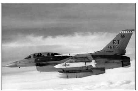
The joint standoff weapon, with high potential for defeating air defenses, is a new stealthy glide bomb with global positioning system accuracy. It can be released well away from SAMs—at a safe distance for airplane and pilot.
