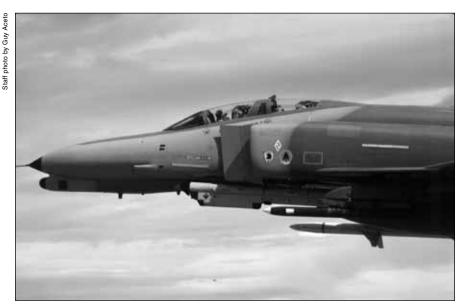
The F-4G was the king of SEAD from Vietnam to the Gulf. The backseater would interpret waveforms and sounds of enemy radars and select threats to attack in order of priority. The HARM Targeting System lacks the F-4G's range and precision, but it automates threat ranking for a solo pilot.
