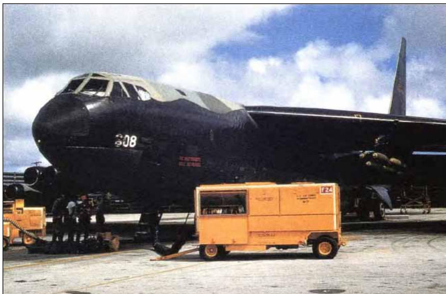
This U Tapao B-52D shows the distinctive black underside favored at the time for night missions. Clearly visible also is the left wing outboard pylon (at right in photo) loaded with extra bombs for Linebacker II missions.
