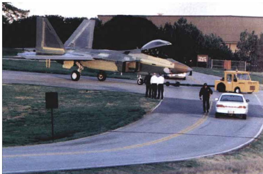
Before its “ghost” paint job, the different colors on the aircraft reveal the various materials—such as titanium, aluminum, and composites—that make up the F-22. Its bulkheads are the largest forged aluminum pieces made.
