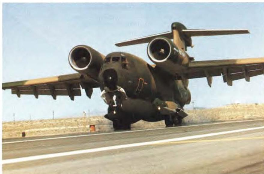
**Blowing engine air over the wings to increase lift has been attempted several times over the years in such aircraft as the Custer Channel Wing (top) and the Boeing YC-14 (above), whose competitor, McDonnell Douglas's YC-15, is an ancestor of USAF's C-17 Globemaster III.**
