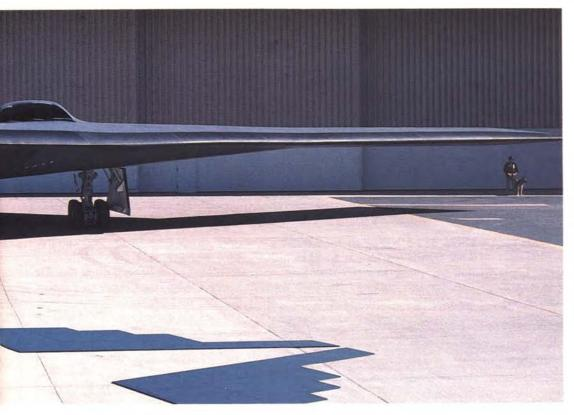
The Northrop B-2 looks particularly sinister in this head-on shot, taken at the rollout ceremonies at Palmdale, Calif. The B-2's wingspan of approximately 172 feet is roughly thirteen feet shorter than that of a B-52. At sixty-nine feet long and seventeen feet high, the B-2 is about six feet longer than an F-15 and the same height as an FB-111.
