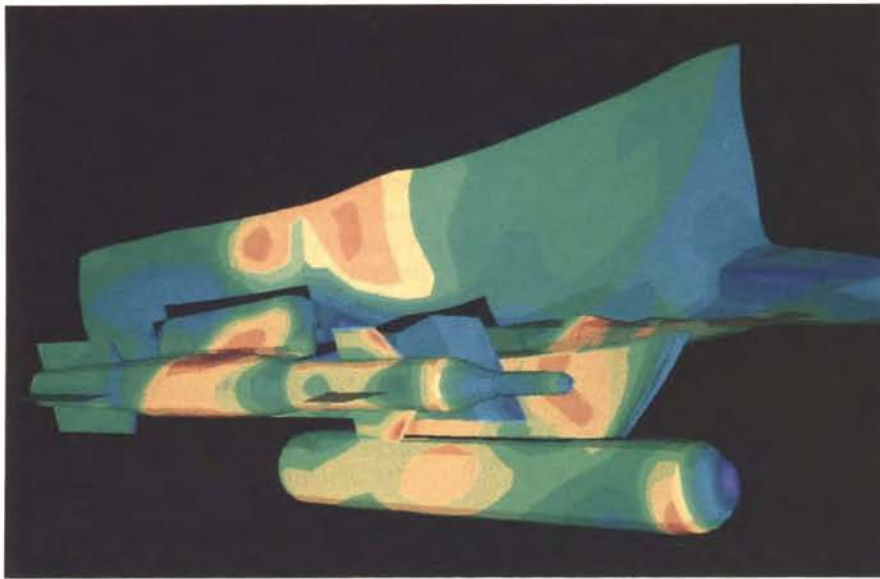
A computer at Wright-Patterson AFB, Ohio, displays Mach number contours on the surface of the F-15E Conformal Fuel Tank, attached LANTIRN pod, and GBU-12. The colors represent changing Mach numbers of the airflow as it follows the shapes of the stores. Cool colors represent low Mach numbers, and warmer colors represent higher Mach numbers.
