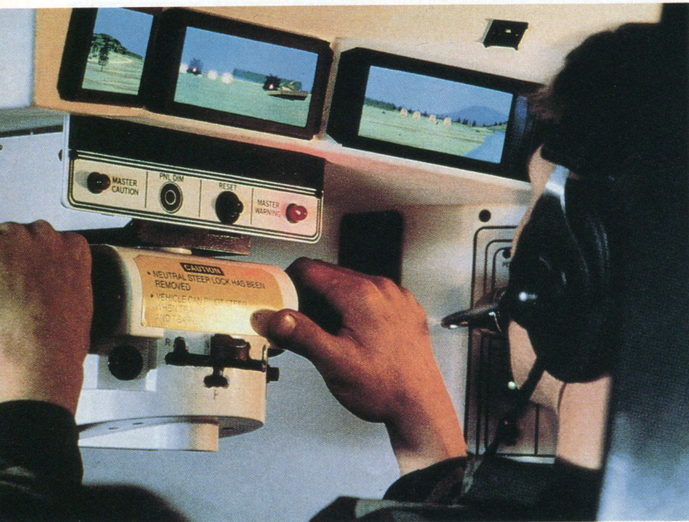
The "tank" simulated here may be the quarry of the "helicopter" shown in the previous photo, even though the users may be at Simnet terminals hundreds of miles apart. Besides the actions of networked "enemy" forces, users must contend with random vehicle failures and other realistic hazards.
