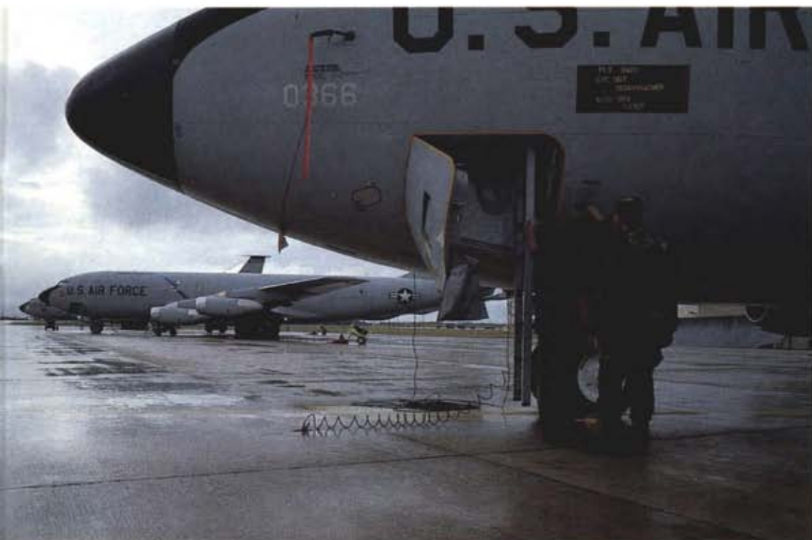
Tankers are an essential adjunct to the bombers. When a plane is on alert, its crew chief (or the assistant) stays on alert with it. Here, the crew chief, with some help from other maintenance troops, finishes preflighting one of K. I. Sawyer's alert KC-135As. The alert aircraft are preflighted every morning, regardless of weather.
