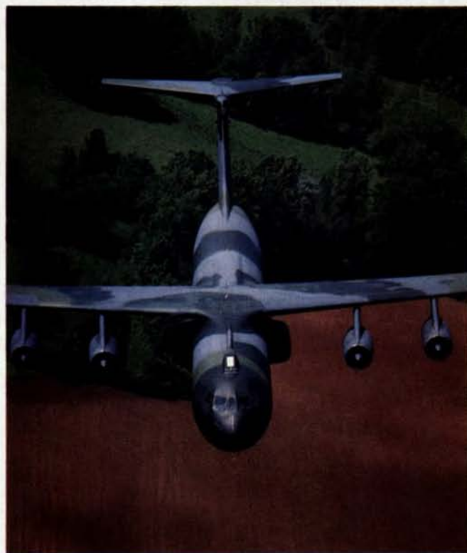
A real force-multiplier was the modification program done to the Air Force's fleet of Lockheed C-141 StarLifters. Adding twenty-three feet to the fuselage of the planes provided a thirty percent increase in volumetric capacity, and an in-flight refueling capacity gave the "StarLizards" global range.
