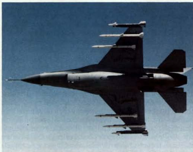
The shape of air defense to come: The General Dynamics F-16 was chosen last year as the Air Force's new interceptor to replace the F-106s and eventually the F-4s now used. This F-16 is armed with two AIM-9 Sidewinder missiles and four AIM-120 AMRAAM missiles, which will replace the AIM-7 Sparrow.
