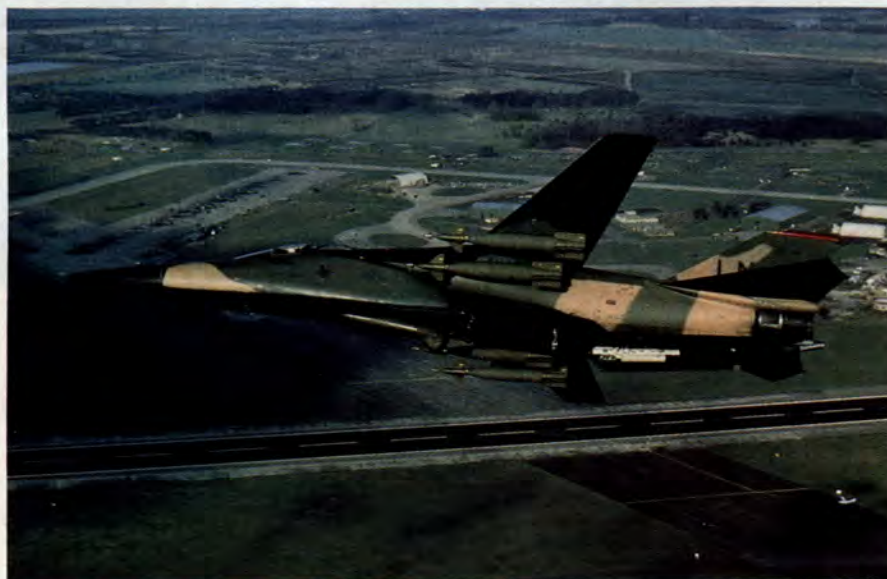
An F-111F from the 48th TFW at RAF Lakenheath, UK, banks away. This F-111 is carrying four Paveway II laser-guided weapons and has its Paveway Tack laser designator deployed under the forward fuselage. F-111s with precision-guided weapons will be used for knocking out critical enemy targets far behind enemy lines.
