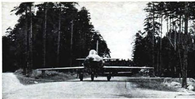
A unique feature of the Swedish air defense system are road bases, especially strengthened sections of the nation's road network designed to serve as emergency wartime bases and flight strips. Above, a Lansen on such a road.
