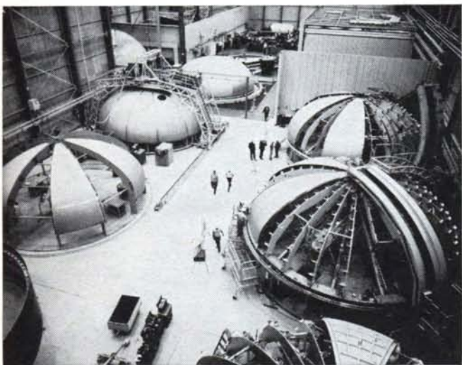
Magnitude of components in moon effort, such as these bulkheads to be used for separation of propellants in Apollo Saturn V booster, shown here under development at North American Aviation, illustrate need for space-age adaptations of successful management techniques of AF ICBM effort.
