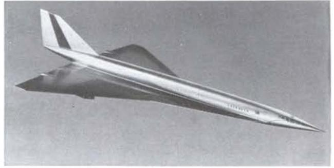
Lockheed proposed a double-delta wing for its supersonic transport (above). This is a Mach 3 aircraft weighing more than 400,000 pounds and capable of carrying 218 passengers more than 3,500 miles. A-11 can play a vital role in development of the SST by serving as systems test bed.
