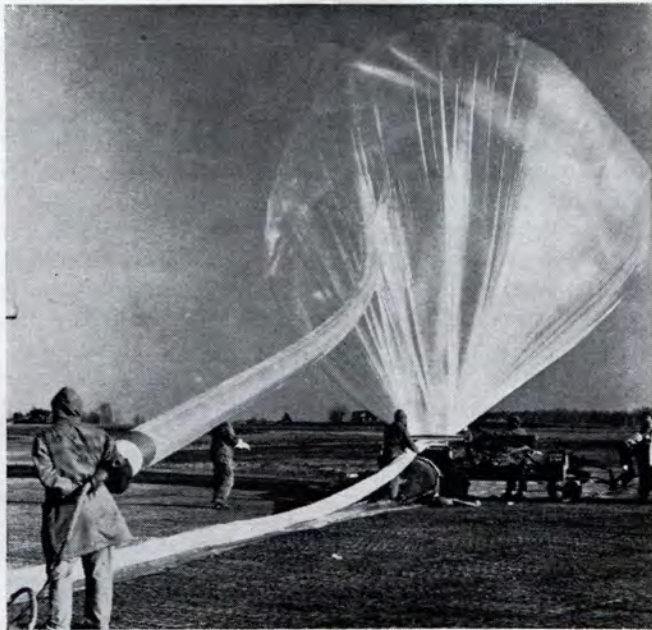
Here balloon in launch arm is being inflated prior to launch. "Bags" are made of polyethylene, are filled with helium. Balloons cost between $750 and $3,500, the helium used in one flight in the neighborhood of $500.
