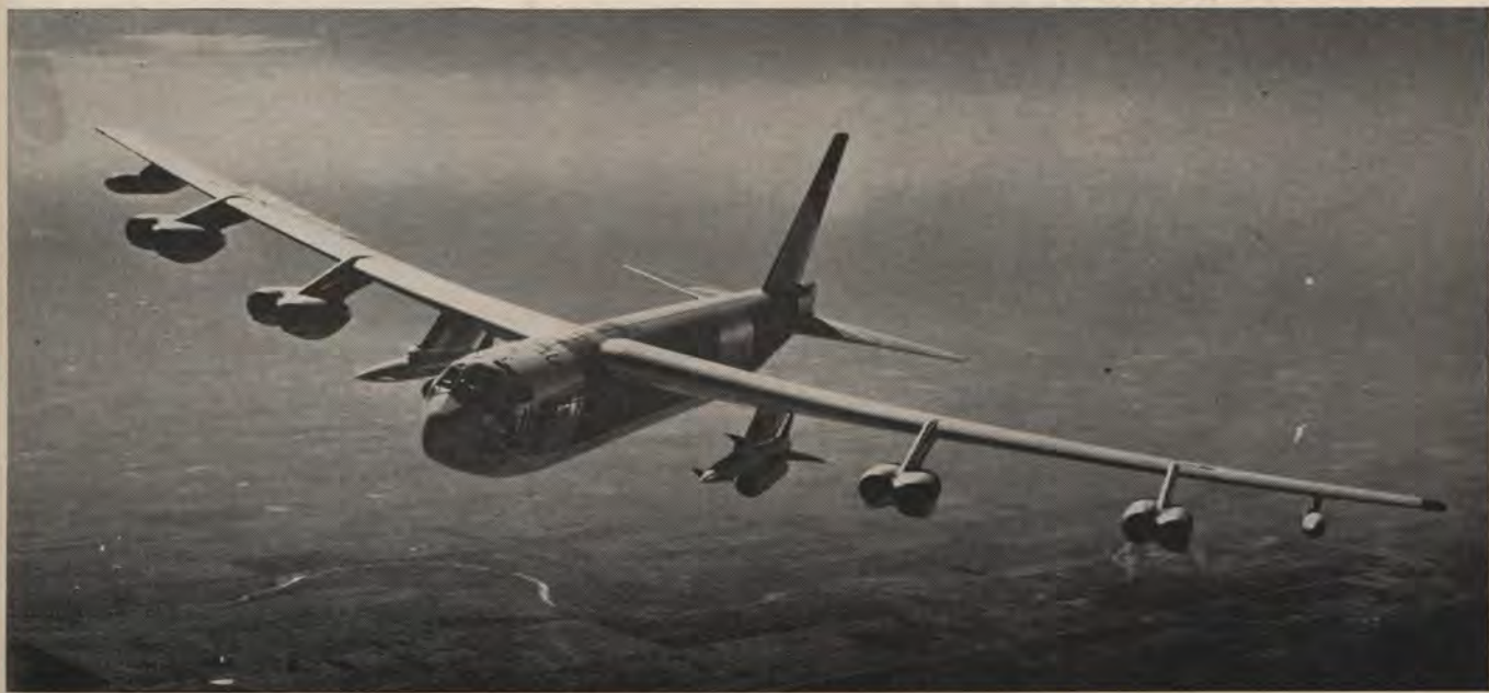
The B-52C, new version of SAC's major current bomber, can carry Hound Dog air-to-surface missiles as well as usual bomb load. The first of the new, turbofan-powered B-52Hs is scheduled for completion sometime early in 1961.
